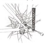
Step 3: Slide the rack legs over the flat brackets. It may be necessary to spread the rack legs to fit.
