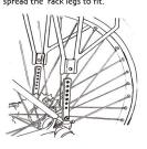
Step 4: Move the rack up and down so the distance from the widest part of your tire to the bottom of the rack is 1" to 2" (25 to 50mm) and parallel to the ground.
