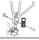
Step 7: Select either the regular or long slotted brackets, whichever is long enough to reach from the rack to the bike while the rack is horizontal. Tip: long brackets can help with smaller bikes. Attach the slotted brackets to the rack using the shorter 6mm bolts and lock nuts. Make them finger tight.
